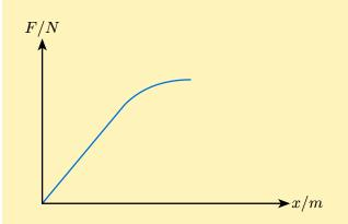
The gradient of the linear section of the graph is the spring constant of the spring.
