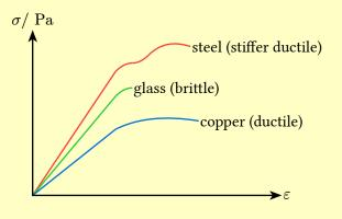
The gradient of the linear section of each graph is the Young's modulus of the material. The area under each graph is work done per unit volume.
