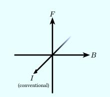
When a wire carries a current perpendicular to a magnetic field, there will be a magnetic force acting on the wire as shown.
